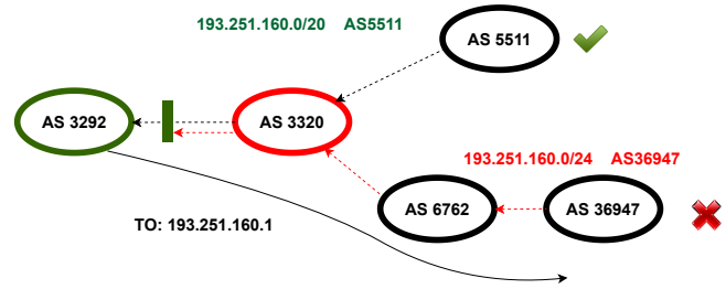
Figure 9: Collateral damage on AS 3292; ROV scores of AS 3292 and 3320 are 92.1% and 0% respectively.
